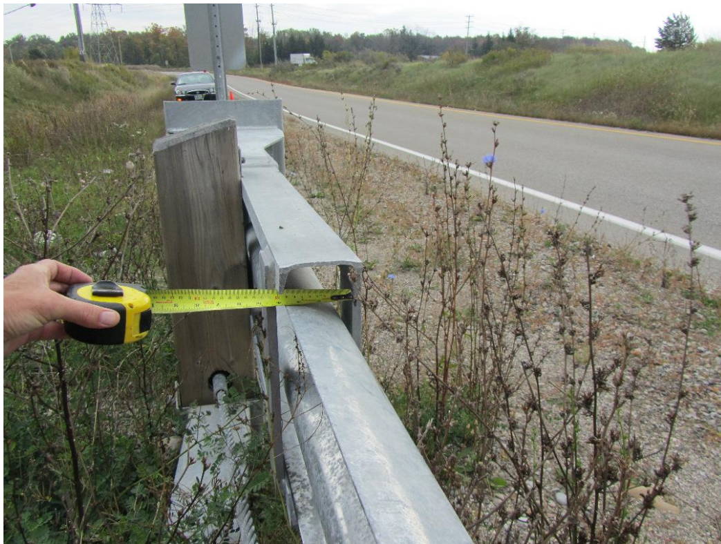
Figure 3: Measurement of channel indicating a width of 4 inches.
