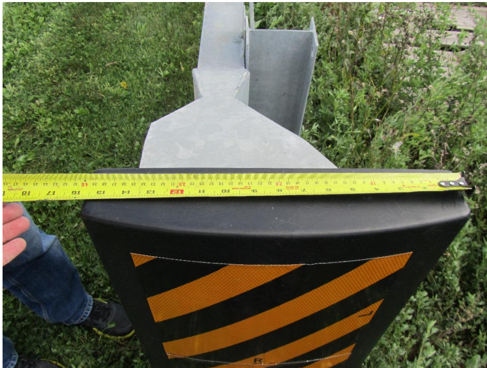
Figure 47: Width measurement (15.5 inches) of end plate cover which is consistent with measurements of other covers
