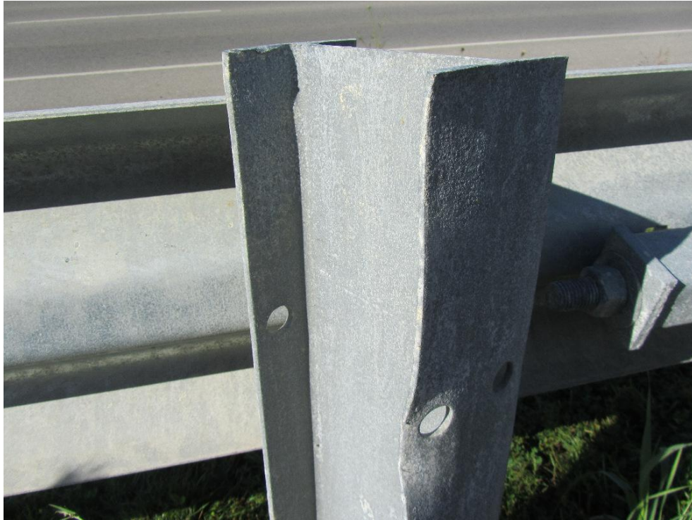
Figure 80: View of deformed status of the anchorage post.
