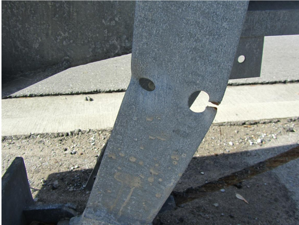
Figure 109: View of buckling and ruptures of the vertical anchorage post just behind the end plate.
