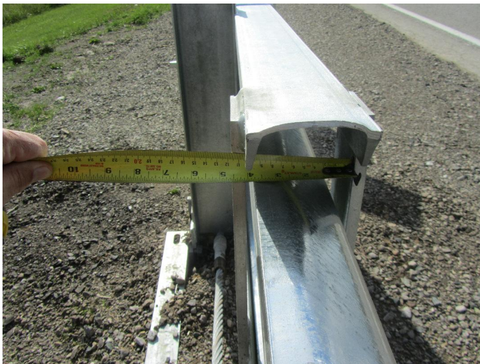
Figure 14: Measurement of channel indicating a width of 4 inches.
