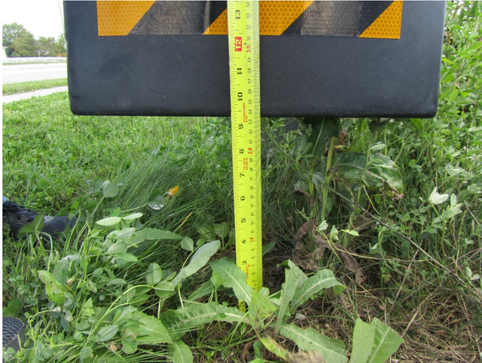
Figure 48: Measurement indicating that the base of the end plate cover is about 9.5 inches above the ground.
