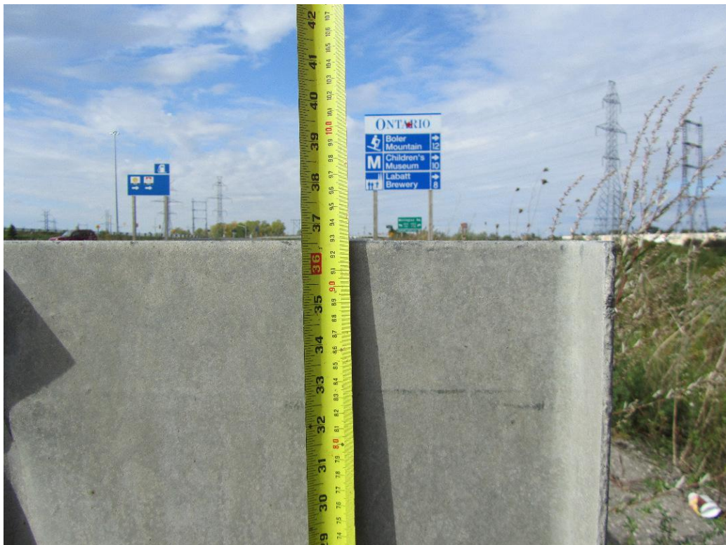
Figure 43: Top of end plate positioned 36.5 inches above the ground, thus the end plate is 28 inches tall.
