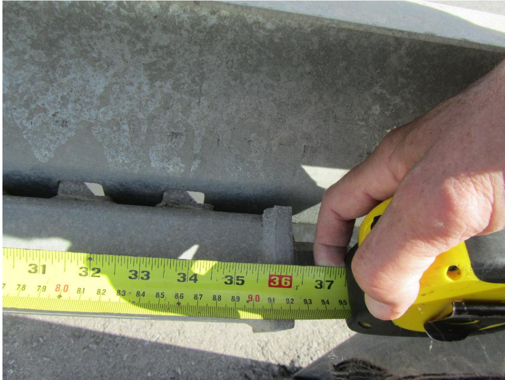
Figure 147: Result of standard measurement indicating a distance of 36.25 inches.
