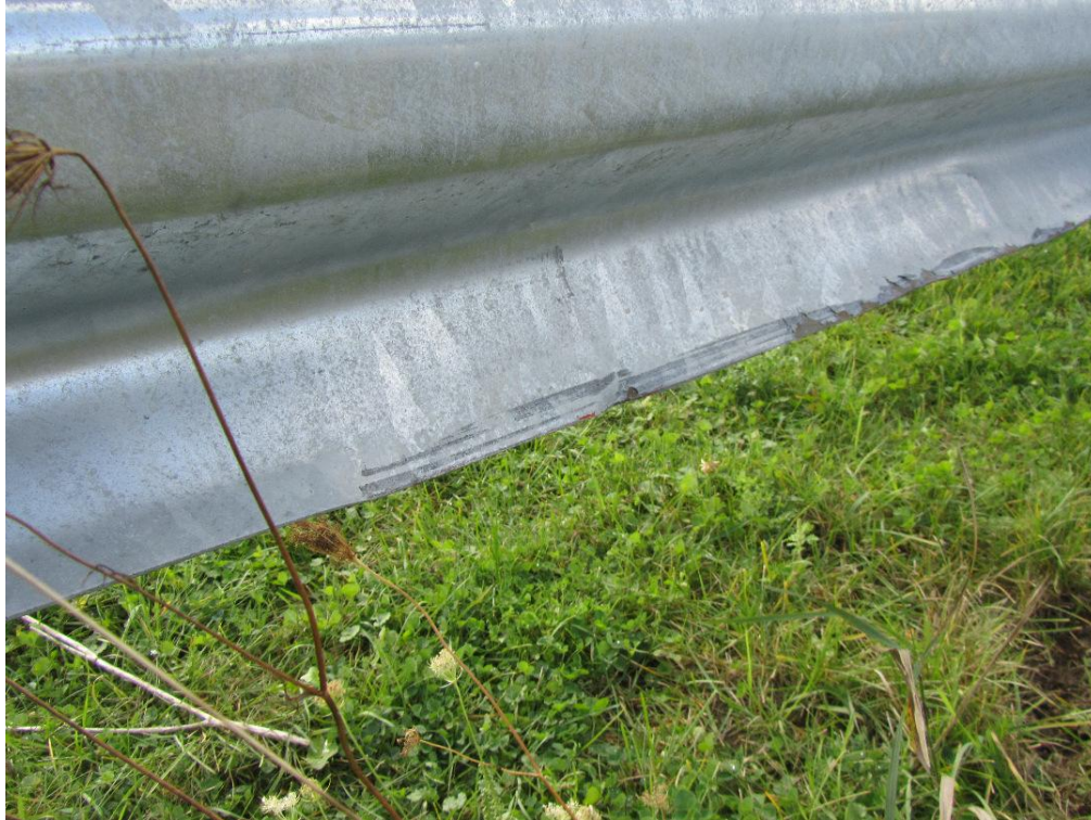
Figure 66: Evidence of scrapes to backside of rail at the location where the rail is deformed.
