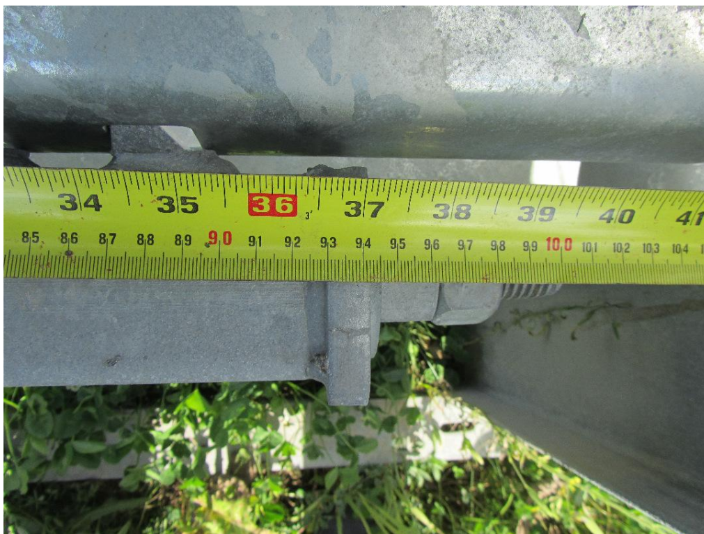
Figure 53: Result of standard measurement indicating a distance of 37.25 inches.
