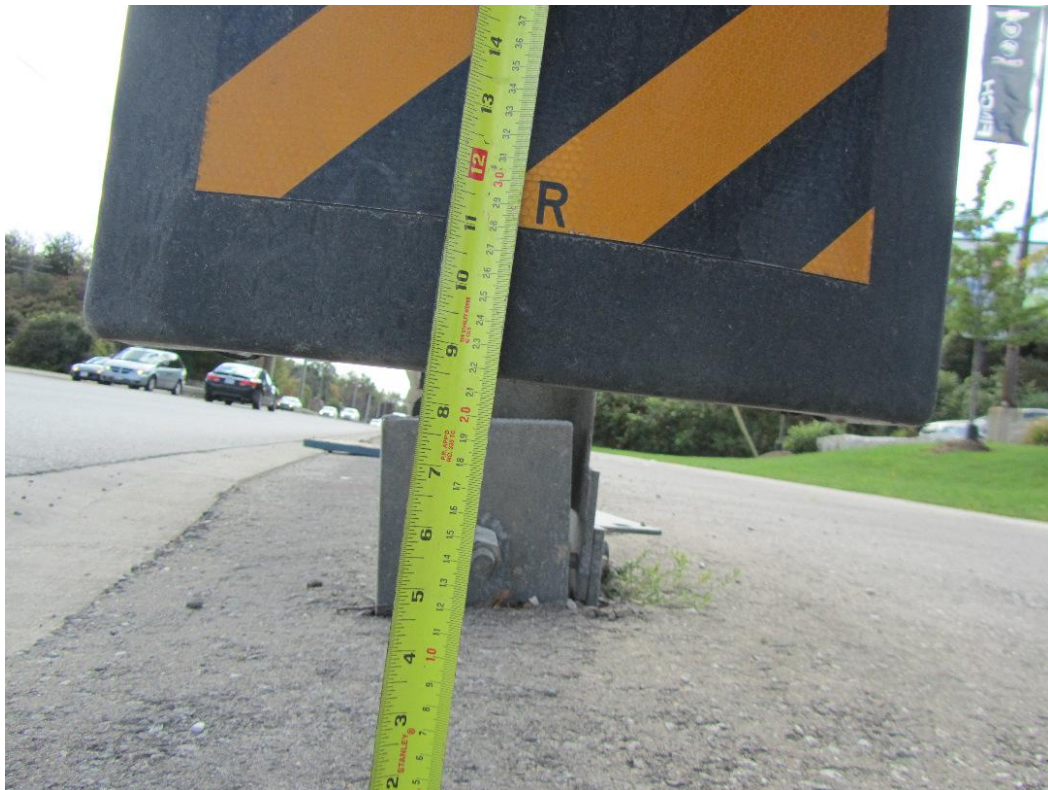
Figure 142: Measurement indicating that the base of the end plate cover is 8.5 inches above the ground.
