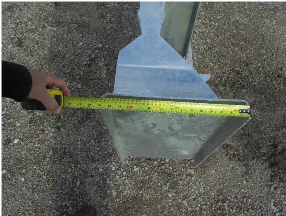
Figure 12: Measurement of front plate indicating a width of 15 inches.
