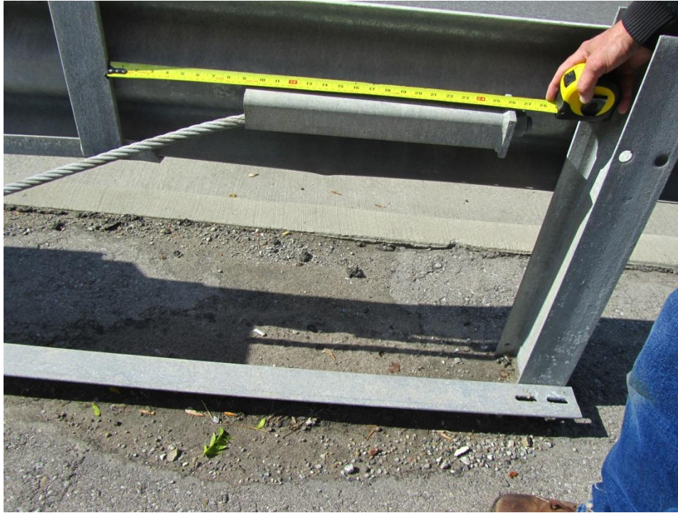
Figure 113: View showing standard measurement being taken to identify the displacement of the end plate along the rail.
