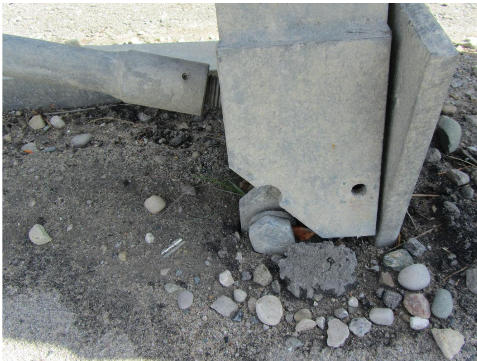
Figure 124: Close-up view of separation at the bottom anchor bolt suggesting that this was a manufactured "tight fit" only and likely designed to separate whenever the end plate sustained a dislocation.
