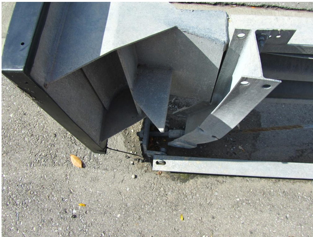
Figure 106: Vertical view of damage near the end plate indicating that the plate has been pushed along the rail, likely due to a previous impact.
