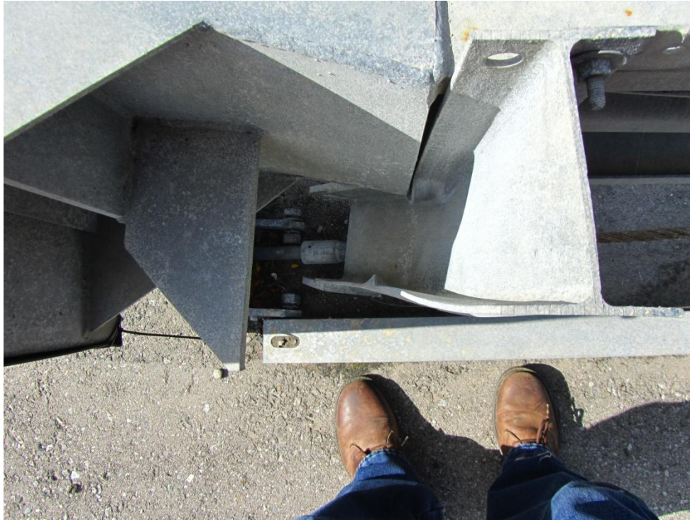
Figure 111: Top view showing how the back of the end plate has made contact with the vertical anchorage post and deformed it.
