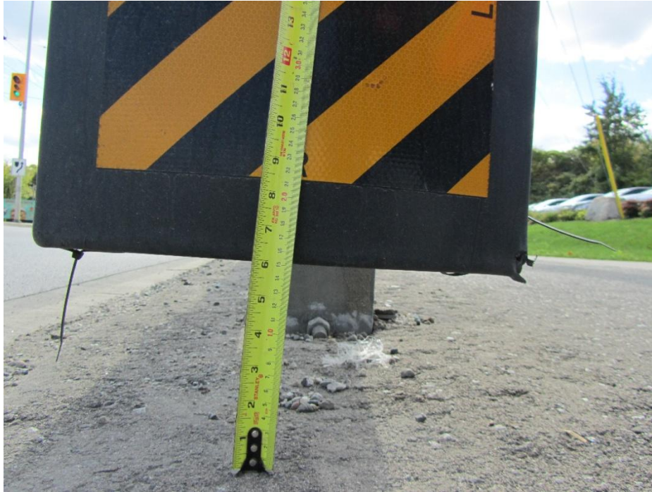
Figure 131: Measurement indicating the base of the end plate cover is 6 inches above the ground.
