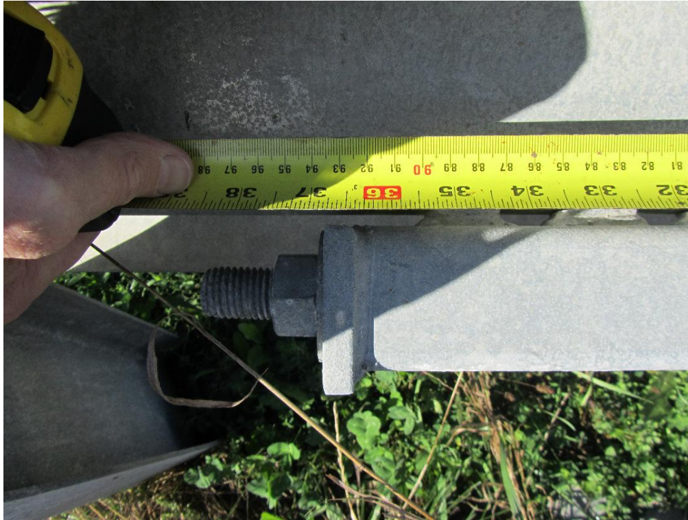
Figure 76: Result of standard measurement indicates a distance of 36.75 inches.
