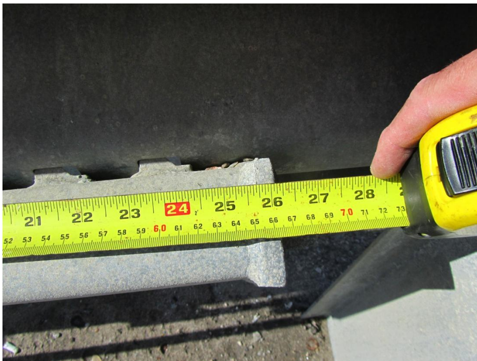
Figure 114: The result of the standard measurement of the 26 inches is about 10 inches shorter than the measurements taken at the undamaged guardrails therefore the end plate as been displaced along the rail by about 10 inches.
